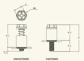
Styled Knob Series Panel Preparation and Installation
